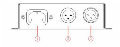
$\texttt{ $\bigcirc$AC100$} \sim \texttt{240V} \text{ power interface } \texttt{ $\bigcirc$DMX signal kalong input interface } \texttt{ $\bigcirc$DMX signal kalong output interface }$
