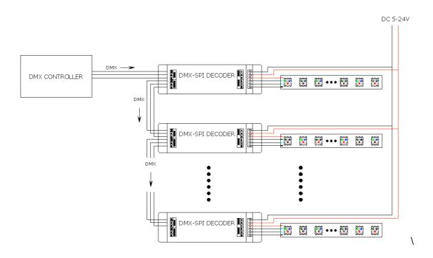
**Double power connect single signal line strip condition:** if the V+ voltage of strip is not the same with controller input voltage and light signal is single, you need to connect another power supply.
