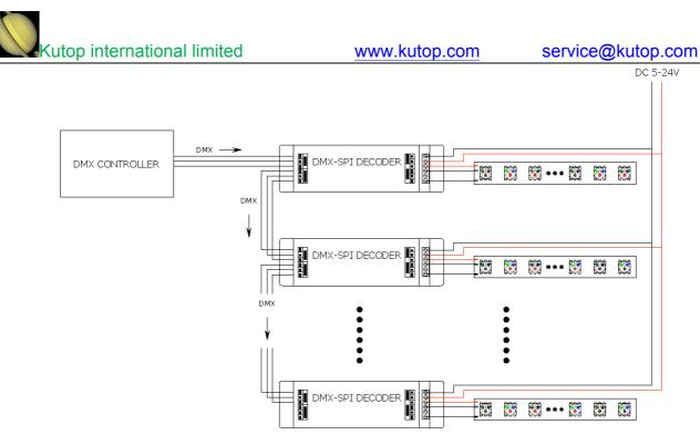
**Single power connect double signal line strip condition:** if the V+ voltage of strip is the same with controller input voltage, and the light signal is double then it can directly connect with the controller V+;
